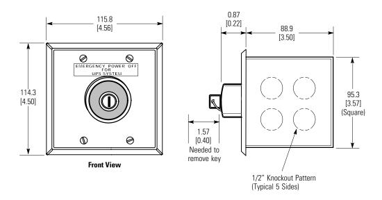
Figure 3-10. Remote EPO Switch Dimensions
